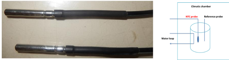
Figure 5 -Negative Temperature Coefficient (NTC) probes and test conditions
